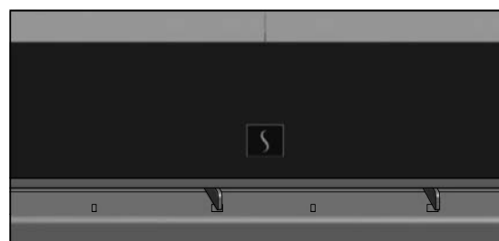
Adjustment of air supply, primary and secondary damper
