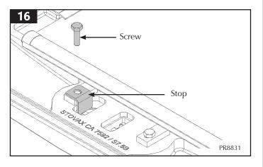
This will stop the control fully closing and a gap of approximately 2mm should be visible, Diagram 17.
