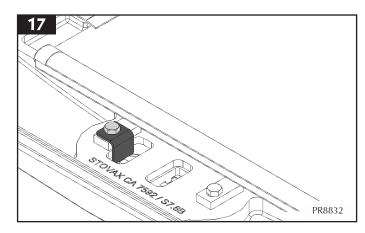
2.10 Refit the fixing screw.
