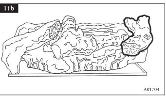
8.8 Place Log E into the groove between Log F (see Diagram 12a) and Log D so that it rests across logs A and D (see Diagram 12b).
