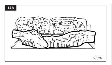
5.7 Put the embers on the burner around the positioned logs. TAKE CARE NOT TO COVER ANY PORTS ON THE BURNER as shown in Diagram 15.
