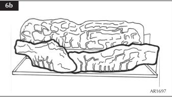
8.3 Put the embers on the burner around the positioned logs. TAKE CARE NOT TO COVER ANY PORTS ON THE BURNER as shown in Diagram 7.
