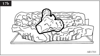
5.10 Position Log B so that the underneath rests in the groove of Log C (see Diagram 18A) and the end is in the corner of the burner (see Diagram 18B).
