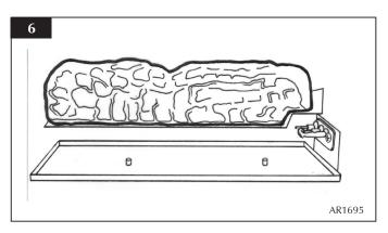
8.2 Place Log C onto the two studs on the burner skin (see Diagram 6a) with charred effect of the log facing forward (see Diagram 6b).
