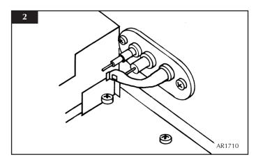
3.5 Remove the two fixing screws from the pilot burner bracket (see Diagram 3).
