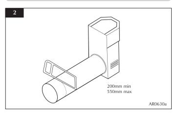
Terminal dimensions:  $395 \times 200 \times 200 \text{ mm}$  (H x W x D) Guard supplied Cut to length as required on site (see Diagram 2).
