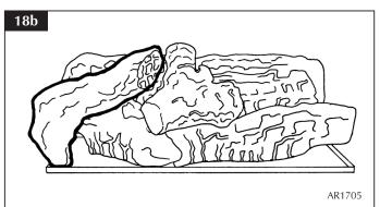
5.11 Put the groove underneath Log F onto Log C (see Diagram 19A) so that F is parallel to the side of the firebox (see Diagram 19B).
