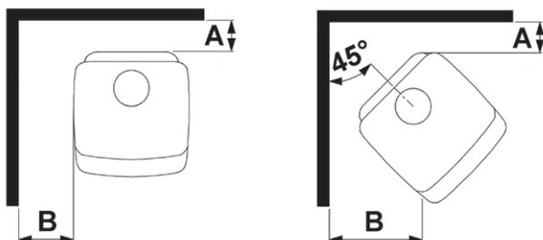
We recommend that the stove be installed at least 10-15 cm from masonry in order to allow heat to circulate and to facilitate the cleaning of the inside and outside of the stove. A layer of wallpaper on a brick wall is normally regarded as non-flammable material.
