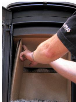
2. Tilt one of the side brick panels and remove it.
