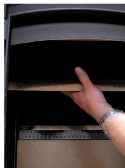
Make sure that the baffles and brick panels are correctly assembled before lighting the stove after cleaning.
