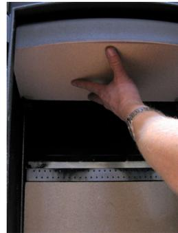
6. Lift the lower baffle down and remove it.
